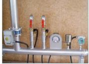
Manometer (Digital & Analog pressure gauge)
